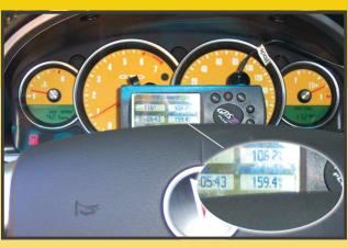
performance related items during a race and taking a line from them, we built a basic system using an infrared sensor mounted in the wheel well that reads each tire temperature on a rotating basis, changing every 10 seconds. Using a baseline of 200 degrees, an alarm system lights a warning light when that temperature is exceeded, giving us the opportunity to slow to reasonable speeds if necessary. It hasn't been, so far.
