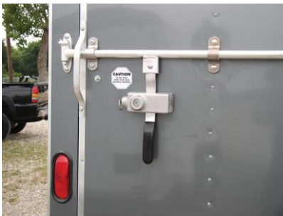
Figure 5 Trailer Door Lock
